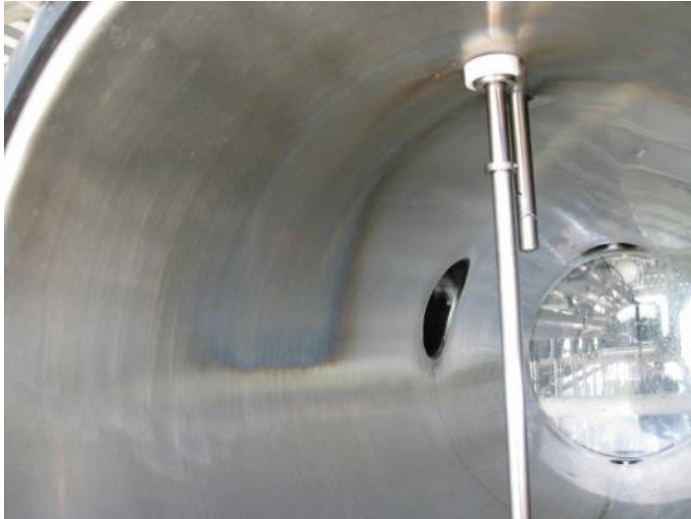
Protein build-up on the interior surfaces of the milking plant
